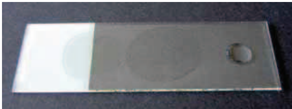
fig. 62: untreated object holder left: linseed oil / middle: isopropanol / right: distilled water
