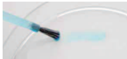
fig. 42: treated surface (72 mN/m)
