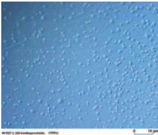
fig. 81: DLC layer with nano scale insitu structure
