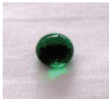
fig. 60: treated cotton (water) hydrophobic
