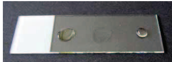
fig. 63: treated object holder left: linseed oil / middle: isopropanol / right: distilled water
