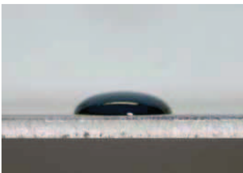
fig. 57: Metal surface untreated
