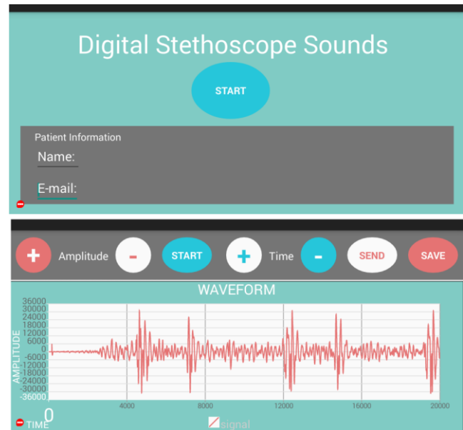
Figure 5. Graphical user interface. The top part shows the initial screen with captured boxes for the patient's name and e-mail. The bottom parts shows the heart sounds displayed on the screen of the phone.
